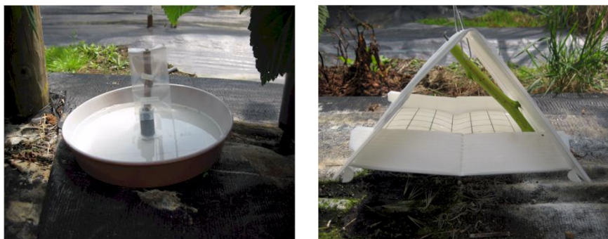
Figure 3. Sachet suspended on dry cane in water trap (left) and primocane wedged in delta trap (right)
